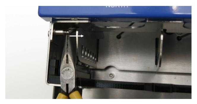
After removing the springs from the top tab remove them form the bottom and take them completely out of the machine.
