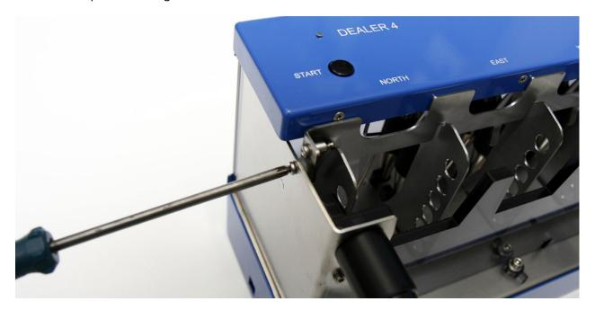
There are two plastic washers on that screw – they can fall down during this operation – it is OK. Find them and put them in a safe place (together with the springs) because they will be needed if the Flip Plate is to be re-attached.
