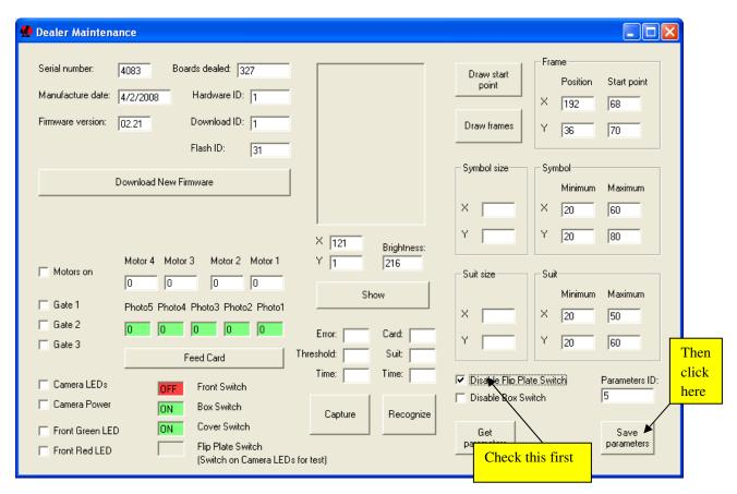
Check "Disable Flip Plate Switch" and then to save this setting into machine click "Save parameters". If parameters are saved correctly following screen appear:
