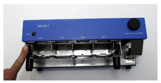
It is not possible to deal with the Flip Plate in the open position. Machine fill detect such condition and display an error:
