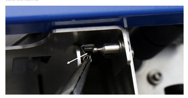
4. Unscrew Flip Plate holding screw from the Left Box Bracket:
