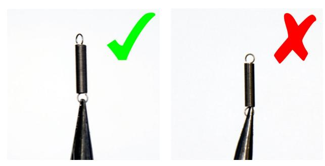
It is important to hold spring on the very end of the pliers tips – otherwise will be impossible to fit end of the spring onto the tab.
