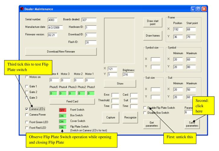
Untick "Disable Flip Plate Switch" and click "Save parameters" to save this change into machine. This step is very important. Without it, the machine will be allowed to deal with the Flip Plate open which will end up in very nasty card jam. It is possible to test Flip Plate switch operation by ticking "Camera LEDs" and observe Flip Plate Switch box while opening and closing the Flip Plate.
