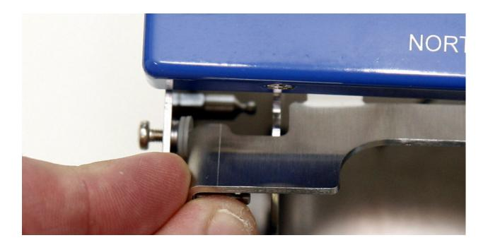
6. Slowly unscrew left screw until Flip Plate slides into position. Navigate Flip Plate until the end of the screw fits into the hole. Then fix the left screw. Plastic washers should stay on the screw during this operation.
