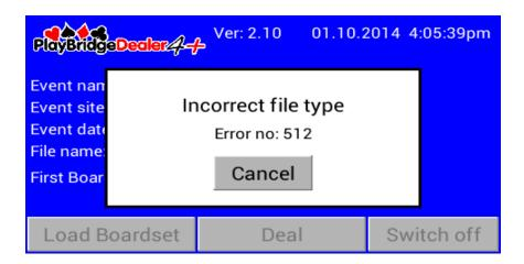
In the case of any loading errors, the Dealer4+ returns to the Main Screen. If the right file is selected but is corrupted or has an incorrect format, more specific information about the problem is displayed - for example:
