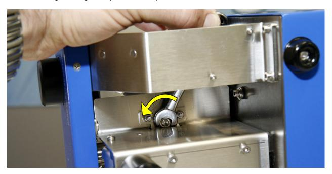
3. Put Feeler gauge blade with desired thickness into Feeder Gap. If blade will not fit (Feeder Gap is too small) rotate card support mushroom anticlockwise (when see from the bottom side) using small flat screwdriver. This makes gap bigger and will allow the Feeler Gauge blade to fit. Some early models (serial numbers from 4001 – 4012 are fitted with a card mushroom without slot for the screwdriver – in such case the mushroom has to be rotated by hand from the top side.
