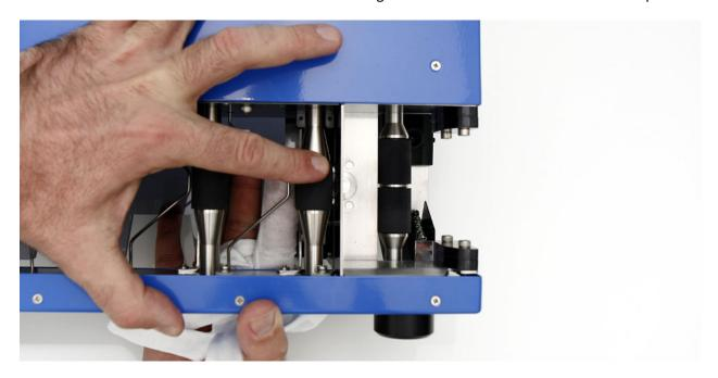
7. After cleaning leave machine to dry, slide Top Cover back (please notice that Top Cover is not symmetrical so needs to be put back in the right direction). The machine is now ready to go.
