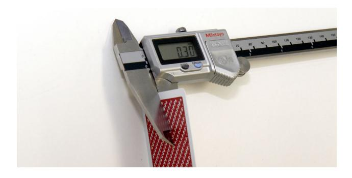
If a vernier caliper is not available it is possible to measure card thickness using standard ruler. To do it get full deck (52 cards), hold them together and measure thickness of all of them. Then divide results by 52. This gives the thickness of a single card.
